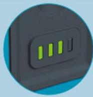
4-stage battery status and state-of-charge display
